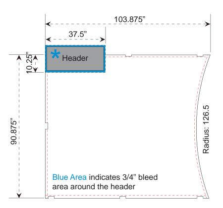
Note: When using a Header with the MOR unit a portion of the graphic will be covered. Please design graphic layout according to suggested location.
